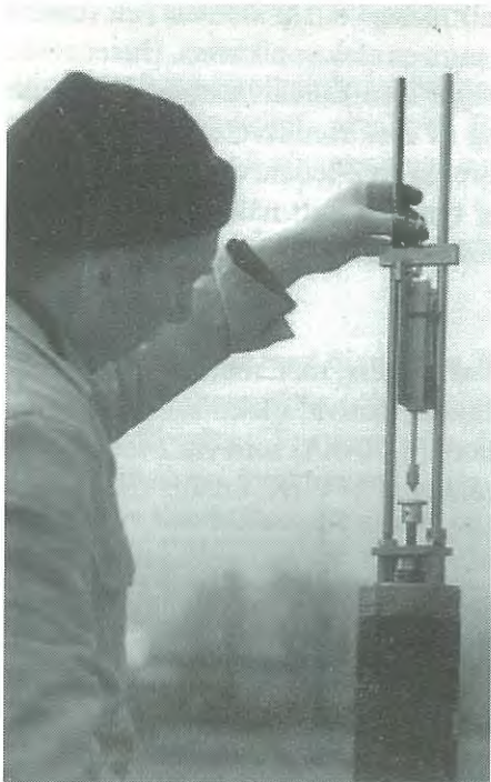
Figure 5.2 SGI automatic settlement gauge (Möller & Åhnberg 1992).
