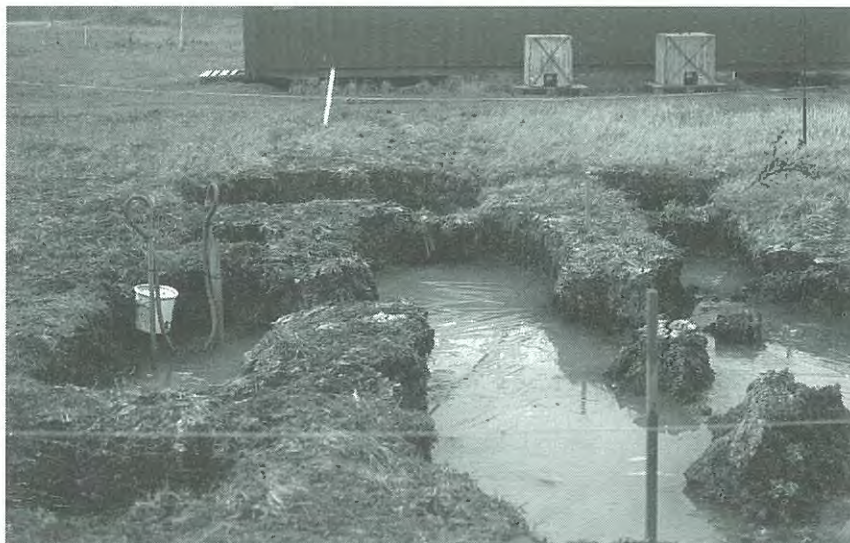
Figure 6.14 Deformations caused by thawing of previously unfrozen soil. (Photo from January 1993.)
